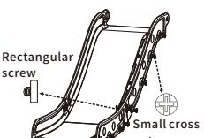
4 Fix the other side of the slide rail and tighten the small cross nut
