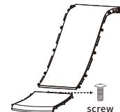
2 Assemble the buffer plate and slideway and tighten the screws
