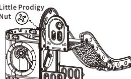
11 Assemble 2-lug platform with star baffles to large side panels
