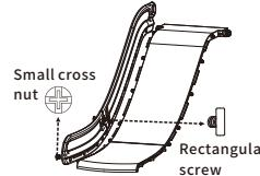
3 Install the slide rail handrail on one side and tighten the small cross nut
