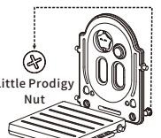
10 Assemble the 2-lug platform with the star baffle and tighten the little prodigy nut
