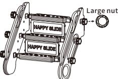
16 Assemble stair railings, treads and stops
