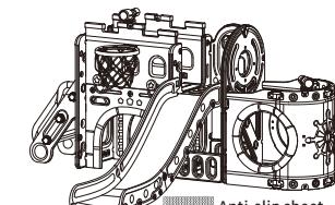
22 Attach an anti-slip sheet to the bottom of the slide and the installation is complete.
