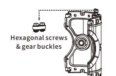
6 Use hexagonal screws and gear buckles to join the two front plates of the boat.
