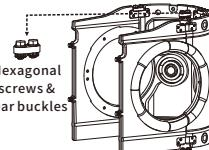
8 Assemble the bow side plate on the other side and tighten the hex screws
