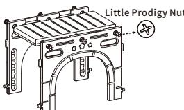
13 Assemble the U-shaped side panels of the aisle to both sides of the aisle platform respectively
