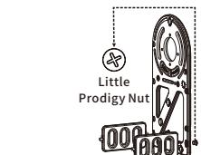
1 Use small prodigy nuts to fix the 3-hole lower baffle to the large side plate respectively.
