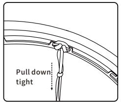
⑤ Tighten the basketball net downwards so that the ropes passing through the hanging holes form a double knot.
