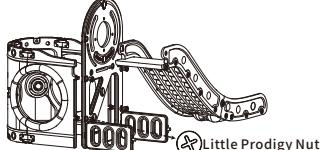
9 Assemble the assembled bow and large side plates and tighten the little prodigy nuts
