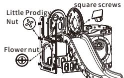
12 Assemble the U-shaped side panel to the other side of the 2-lug platform
