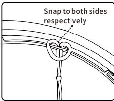
④ Snap the basketball net into the grooves on both sides of the hanging hole
