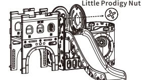
15 Connect the assembled aisle to the slide and tighten the little prodigy nut
